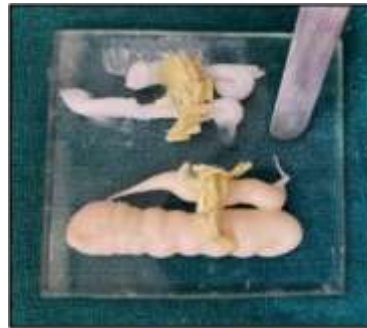
Figure 5: Aramid fibre mixed with bas and catalyst of BAC
