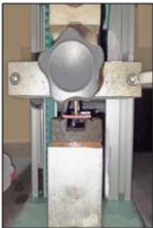
Figure 6: Flexural Strength testing by 3-point bend test
