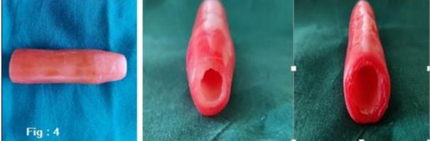
4. Investing the wax mould in gypsum investment material (Dental stone Type III- Asian Chemicals, Rajkot, India ) in two compartments such that the resin will not overflow into the passage. As the dimension of the specimen exceeds the dimension of a dental flask, the investing procedure is carried out in a kidney tray which can accommodate the length and width of the specimen. A layer of petroleum jelly (Jyothi laboratories, Bengaluru, India) is applied for easy separation. (Fig 5)
