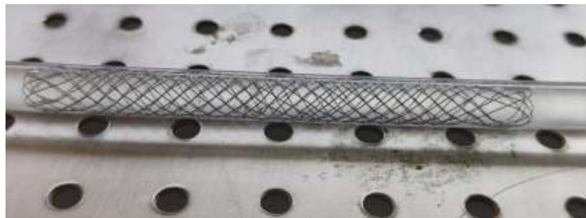
Figure.09 Stent regaining original shape after deployment
