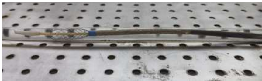
Figure.08 Precise catheter navigation into intended location in curvature model
