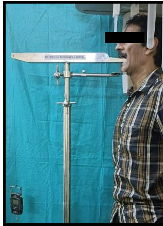
Figure 8a and 8b: Measuring of retentive force using the specially designed apparatus & cephalostat. a Frontal view. b Profile view
